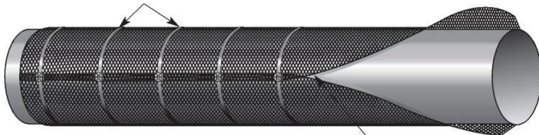
The Denso Stoneguard being overlapped by 150mm.
